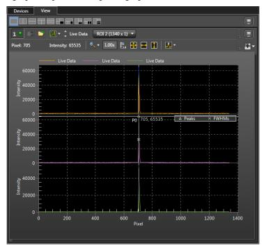
Figure 21. Spectrometer Alignment: After Rotational Alignment
